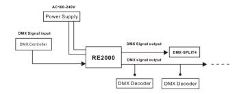
\*At the end of the wiring, we should connect a DMX signal finalizer
